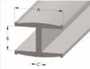
H-profile Oval Beaded (C = 1,2 mm) bead radius = 0,3 mm
